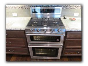
When the oven thermostat alarms sounded, the thermostats for the ovens were found to be inaccurate. The temperature was observed to be greater than a 25 degree difference, either cooler or warmer, of 350 degrees, as measured by a detached thermometer. Recommend further investigation and or repair by a professional appliance technician.
